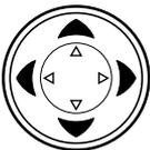
Use the four-directional Cursor key to move the on-screen cursor up, down, left, right.
